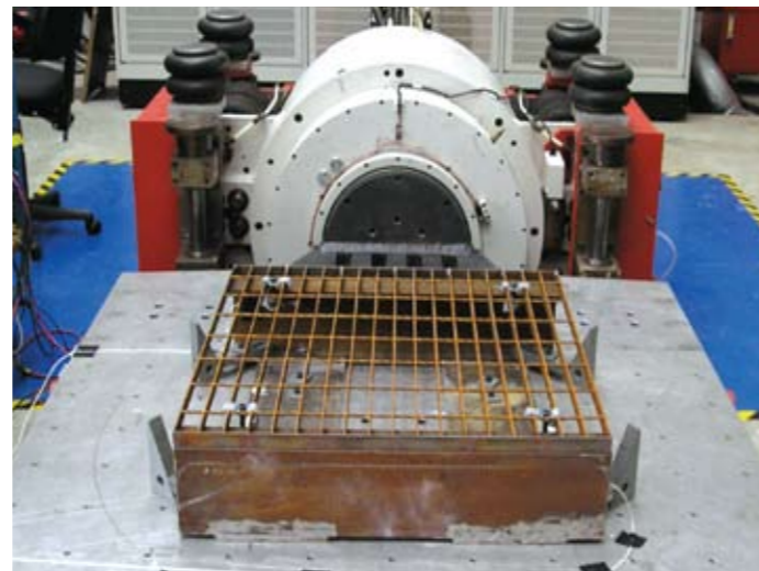
Horizontal Axis Test
