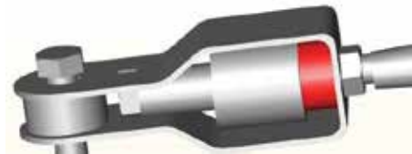
Figure 20 - Un-tensioned Tension Indicator
