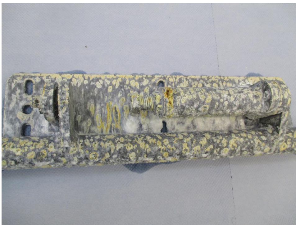
Fig 4: Photograph showing the condition of the Sample after 240 hours Salt Spray Test
