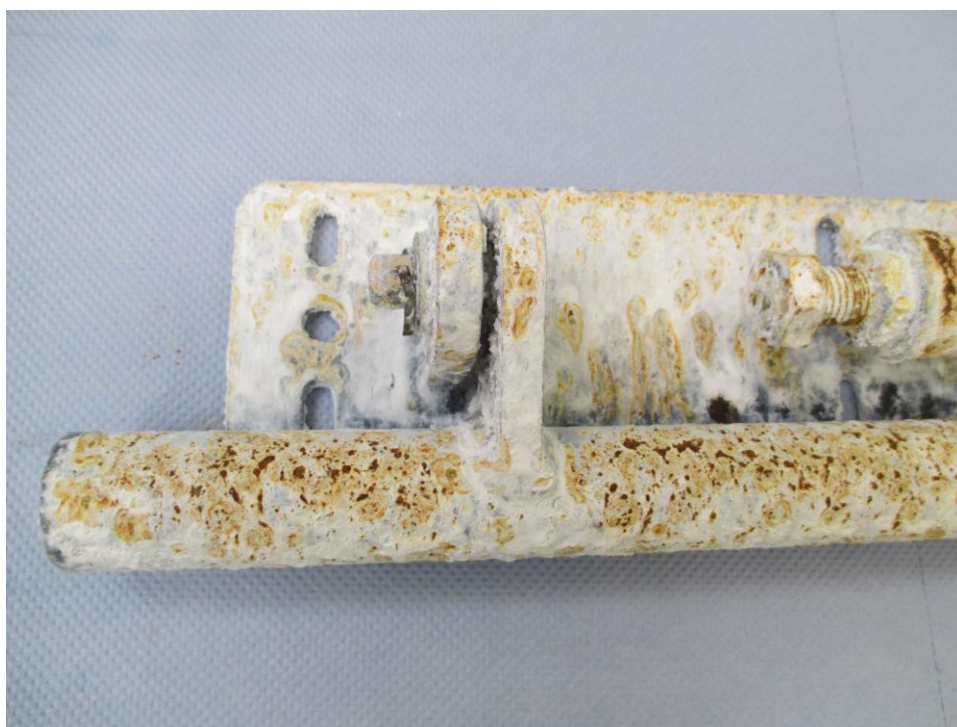
Fig 7: Photograph showing the condition of the Sample after 672 hours Salt Spray Test
