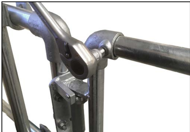
F. Disconnect the tubular gate from the hinge assembly by loosening the top & bottom cast clamp grub screw, using a hex head socket as shown.
