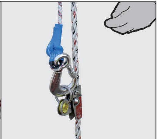
k. Position the Rescue Kernmantel Rope over the Edge Protector. Now carefully lower the Rescue Rope Grab down towards the casualty. The Rescue Rope Grab device will descend easily under gravity to the “D” ring of the casualty’s harness.
