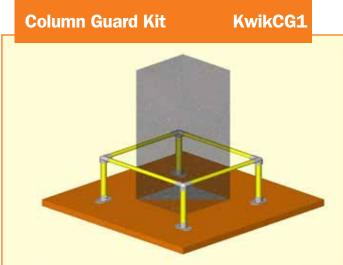
**KwikCG1** is a Column Guard manufactured from 48.3mm diameter galvanised steel tube, 800mm square with four uprights and flat fix baseplates.
