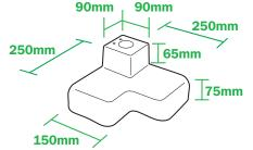
PVC BASE - 250-6 Recycled PVC base provides the support for the Vertical Standards.
