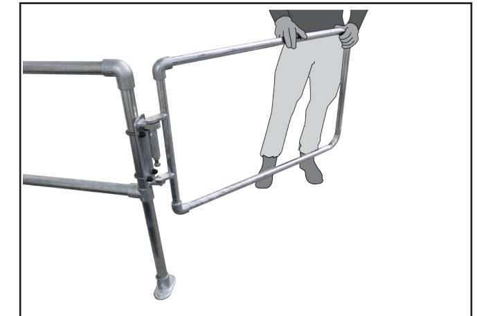
L. Manually open the gate at 45 degrees from its closed position.
