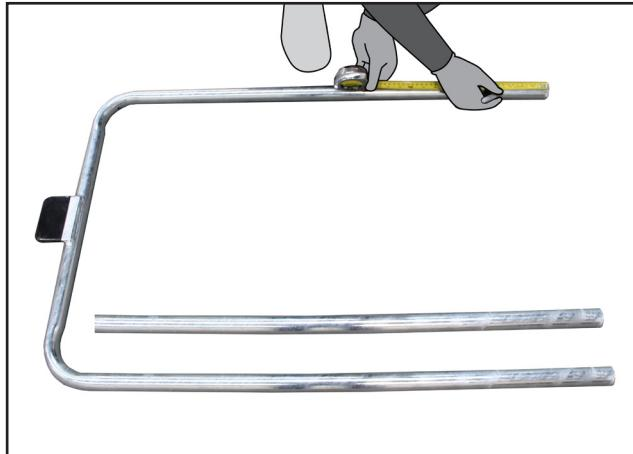
H. Measure the distance recorded in point (f) above and mark the gate top and bottom tubes, and mid rail as shown.
