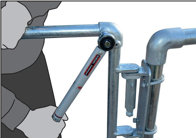
**GB** - G. Disconnect the tubular gate from the hinge assembly by loosening the top & bottom cast clamp grub screw using a hex head socket as shown.
