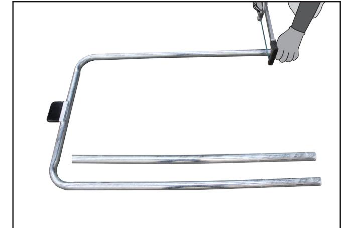
I. Using a hacksaw or similar, carefully cut through the top, bottom tubes and mid rail as shown. For galvanised assemblies, spray with Galvafroid or similar to prevent corrosion.
