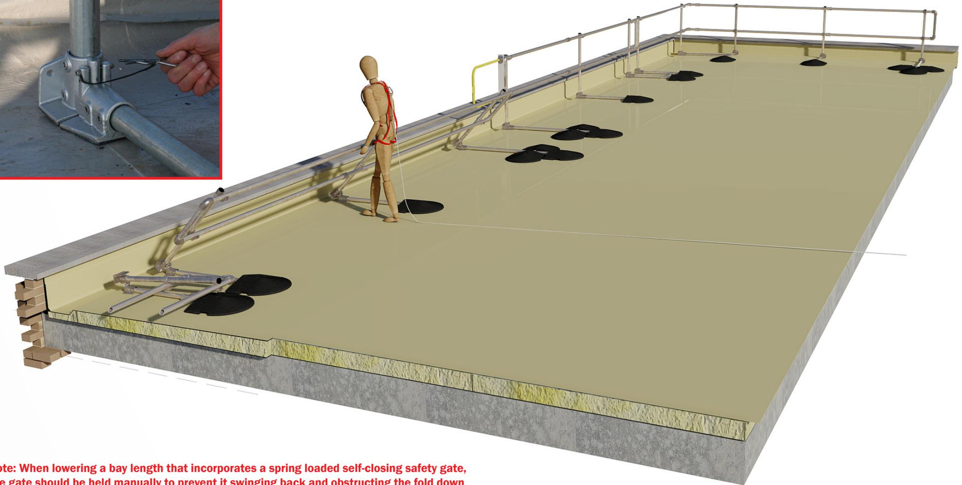
**Note: When lowering a bay length that incorporates a spring loaded self-closing safety gate, the gate should be held manually to prevent it swinging back and obstructing the fold down procedure.**
