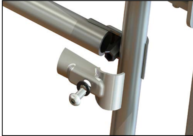
M. Add clamp onto other end of mid rail, clamping onto the gate upright. Use 6mm hex head socket to tighten supplied M10 bolts into coupling nut.
